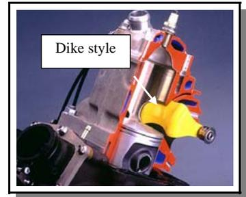
The movement of the valve can be controlled in several differing ways. Some designs use exhaust or cylinder pressure to activate the valve while others use an electro/mechanical method. A third style uses a direct cable or mechanical linkage to operate the valve. Though each design has its own benefits and disadvantages, all suffer from a similar problem. That problem, is that they all require periodic maintenance.
