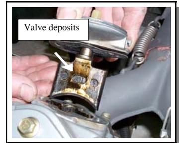
One should keep in mind that the level of force available to activate these valves is minimal. Even moderate restriction due to deposit formation can render the valve in-operable. In order to maintain peak performance, periodic maintenance is required. Within the snowmobile industry, some recommend that valve maintenance (cleaning) be performed as frequently as after every 500 – 1,000 miles of operation.
