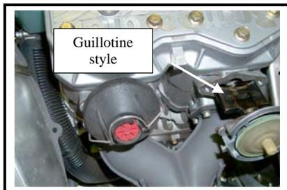
closed position, covering a portion of the exhaust port. In this position, low and lower speed performance is maximized. As the engine reaches higher operating speeds, the valve is retracted creating a larger exhaust port. The end result is a maximization of high-speed operation without sacrificing low end and mid-range performance.
