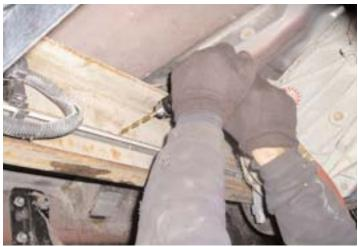
Drilling holes in the frame to install the mounting bracket. The holes were center-punched using a transfer punch to get the exact locations.
