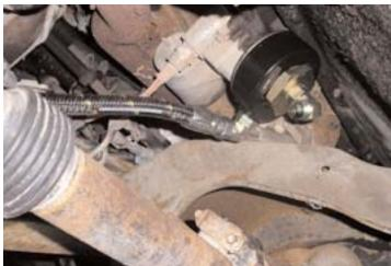
Engine adapter with one of the hoses installed.
