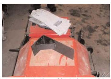
The mounting bracket that was fabricated for this installation.
