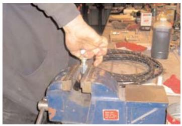
Installing the hose-end fittings. Note that the tapered adapter fitting in the above photo was lightly oiled so that it would install and fit properly in the hose during the tightening procedure.
