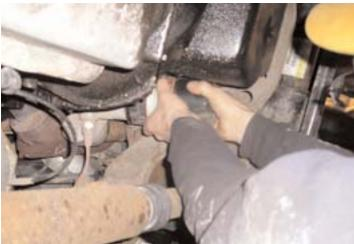
Removing the old full-flow filter.
