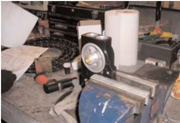
The valve block in the vice being prepared for adapter installation. Note that aluminum vice jaws with rubber cushions were used to prevent damaging the valve block.
