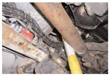
Hose route on the driver's side inner frame rail. It was ziptied and secured so that it cannot interfere with the front driveshaft. There must be a small amount of slack left in the hose to allow for engine roll.
