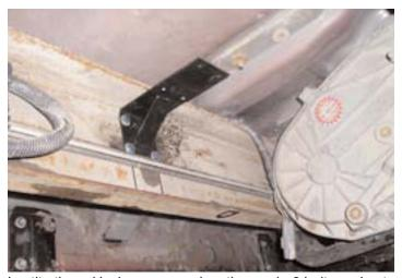
Loctite thread locker was used on the grade-8 bolts and nuts used to bolt the bracket to the frame.
