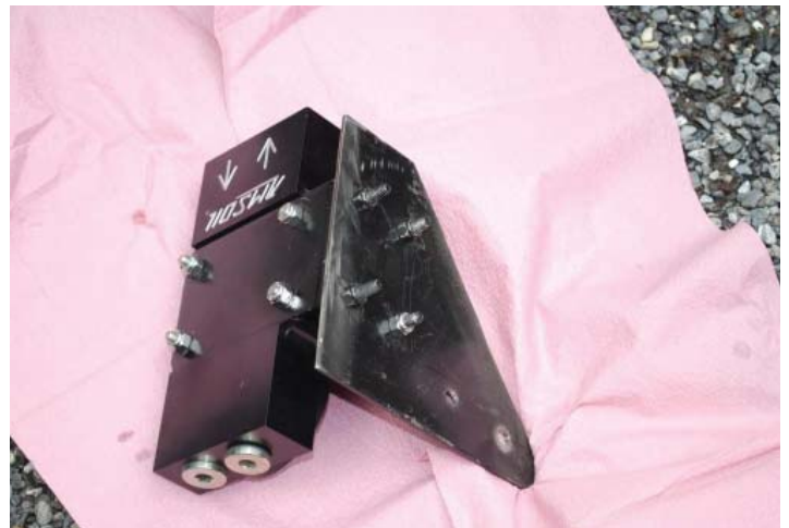
A self-fabricated bracket holds the filter manifold.
