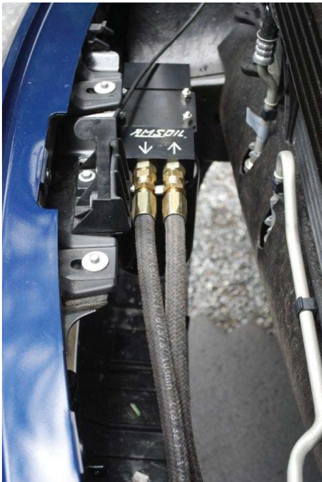
Installing the Dual Remote Filtration System (BMK23) behind the front bumper leaves enough room for a 10" by-pass filter.
